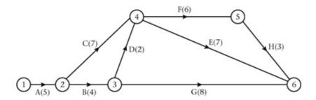
A project is modelled by the activity network shown above. The activities are represented by the edges. The number in brackets on each edge gives the time, in days, taken to complete the activity.
